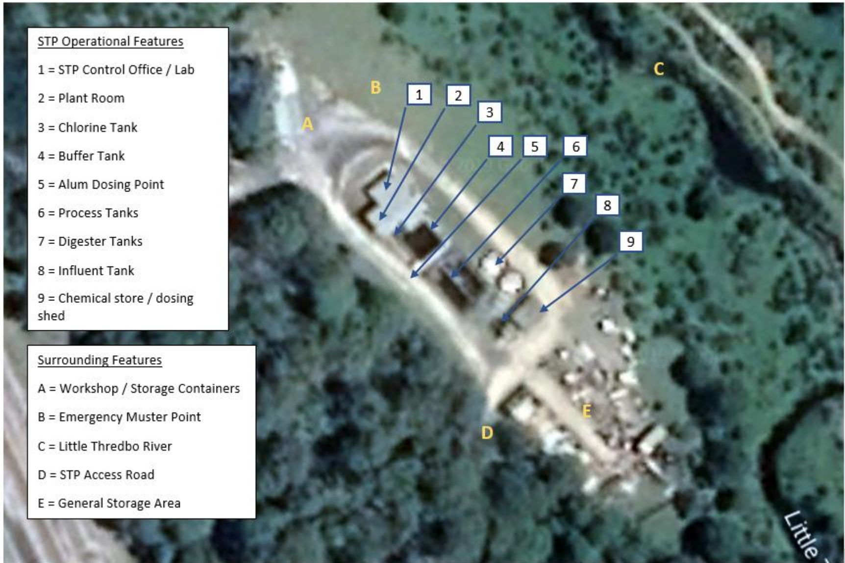
Figure 9.3 STP Operational Features
